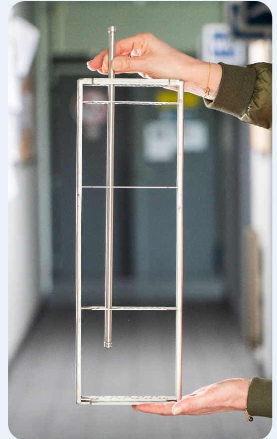
Gamma technology uses cobalt-60, a radioactive source safely encapsulated in double-walled stainless steel, often referred to as a 'pencil' (here empty).
